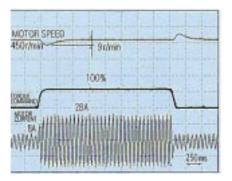
Quick response to rapid changes in load (Speed recovery characteristics upon impact load)
