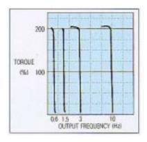
High starting torque at low speeds without PG [Speed control range 100:1 (1000:1 with PG)]
