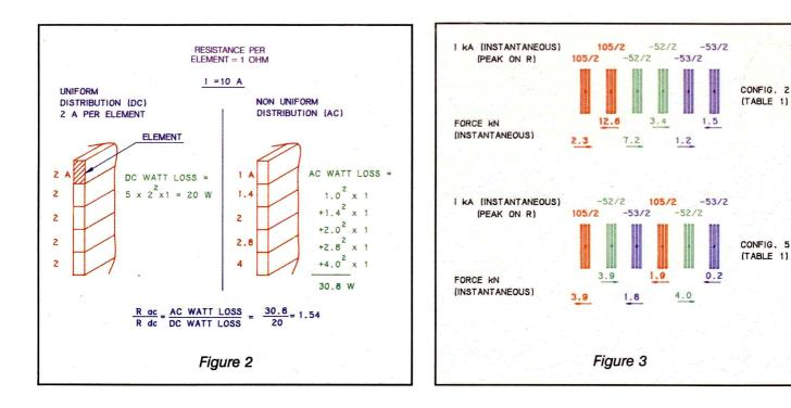
2, effective resistance for middle phase is less than half. Therefore, ampacity would be more by around 35 to 40% for aluminium and 40 to 45% for copper or in other words, the losses will be less in the same proportion.
