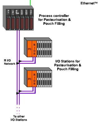
A typical dairy automation system. The entire process is fully automated from reception of fresh milk upto milk dispatch using process controllers, 'Panorama' operator station, process instrumentation and MIS system communicating over plant wide Ethernetô network.
