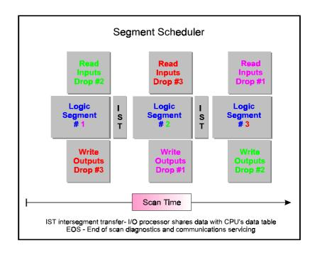
The soft configurable Segment Scheduler™ in **Quantum** process controller complements the high performance of the network by interleaving I/O servicing and logic solving through parallel processing to provide the highest system throughput.
